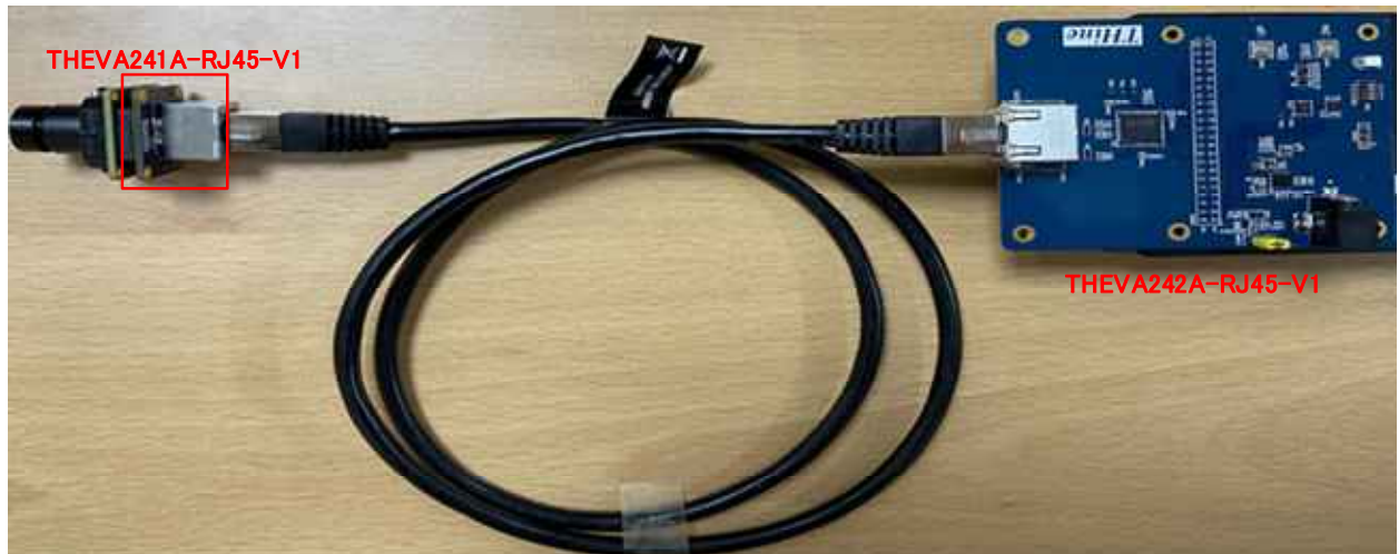
Figure 2 THEVA241A-RJ45-V1 and THEVA242A-RJ45-V1 connection
