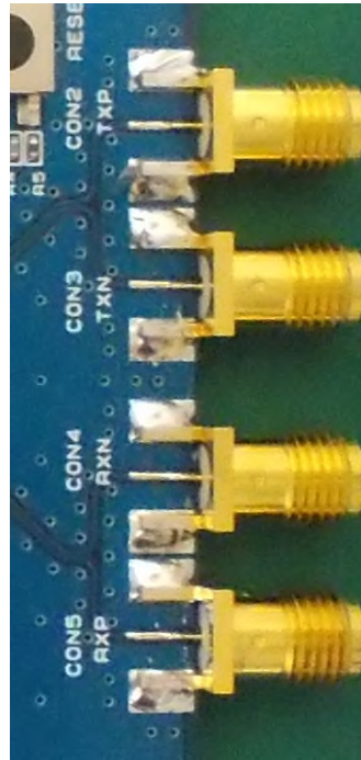
Figure 6 THEVA251-SMA-V3 High Speed CML I/O connector
