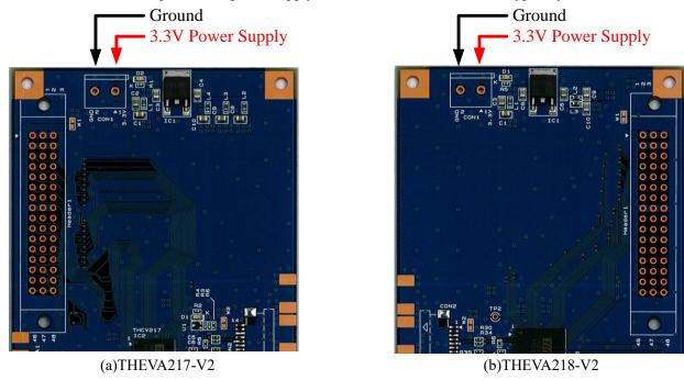
Figure 2 Power Supply for Evaluation Board
