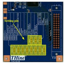
Figure 8 Position of Function Setting Pin
