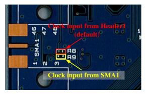
Figure 10 TTL Clock Input Connector Select
