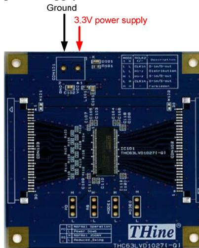
Figure 2 THEVA1027-V2 power supply for evaluation board
