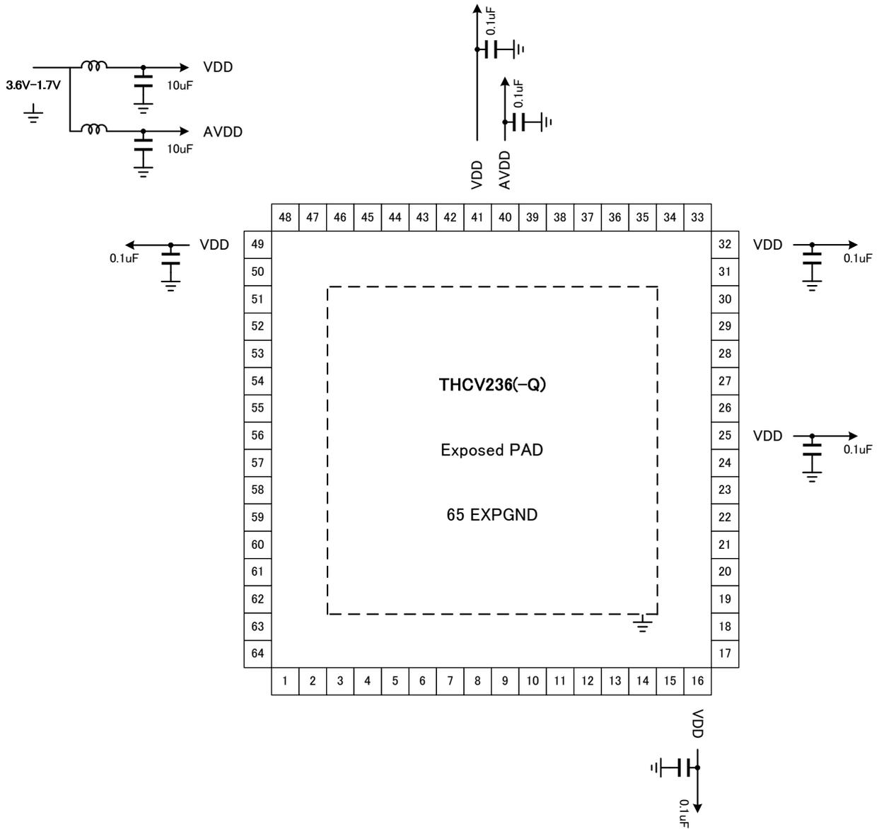
**PCB layout guideline between VDD (41Pin) and AVDD (40Pin) for THCV236(-Q)**
