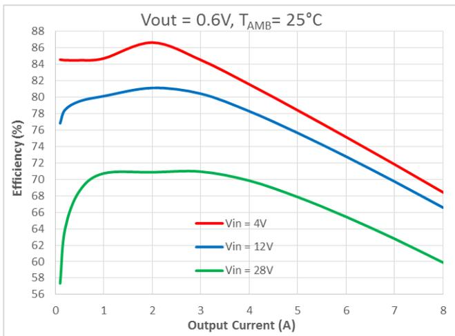
Fig. 11 Efficiency vs Output Current (V<sub>OUT</sub>=0.6V)
