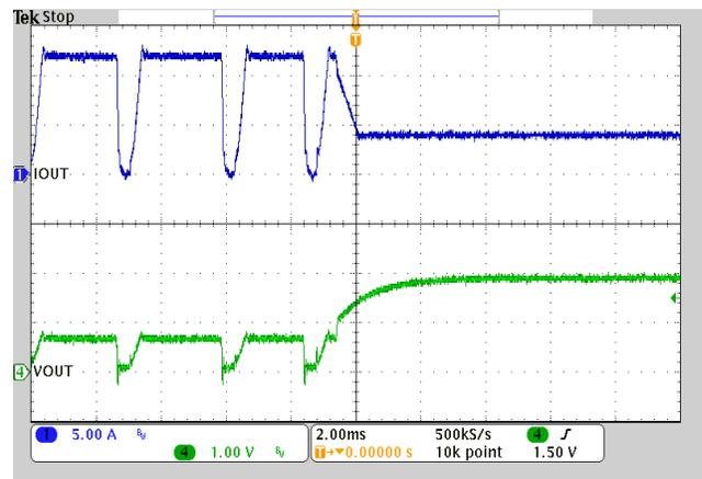
Fig. 28 Recovery from overcurrent
