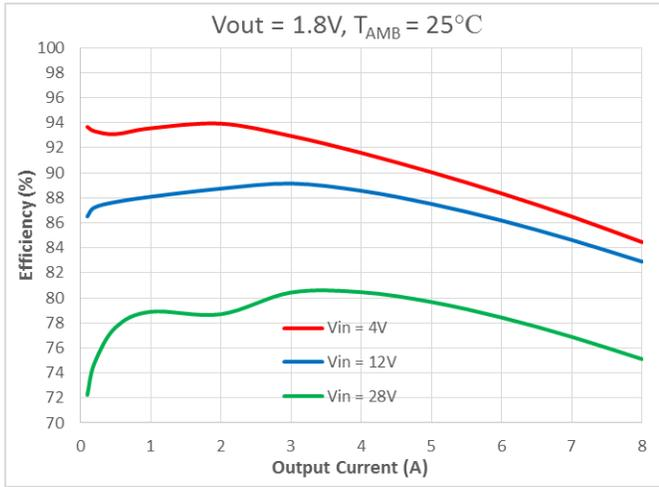
Fig. 7 Efficiency vs Output Current (V<sub>OUT</sub>=1.8V)
