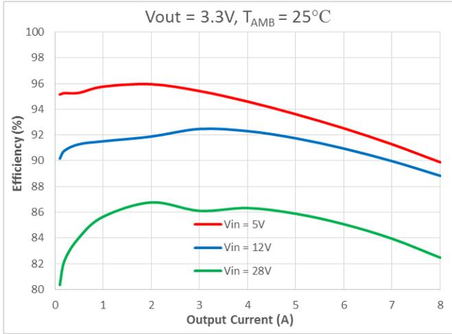
Fig. 5 Efficiency vs Output Current (V<sub>OUT</sub>=3.3V)
