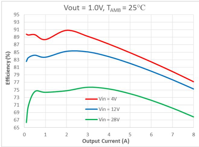
Fig. 9 Efficiency vs Output Current (V<sub>OUT</sub>=1.0V)
