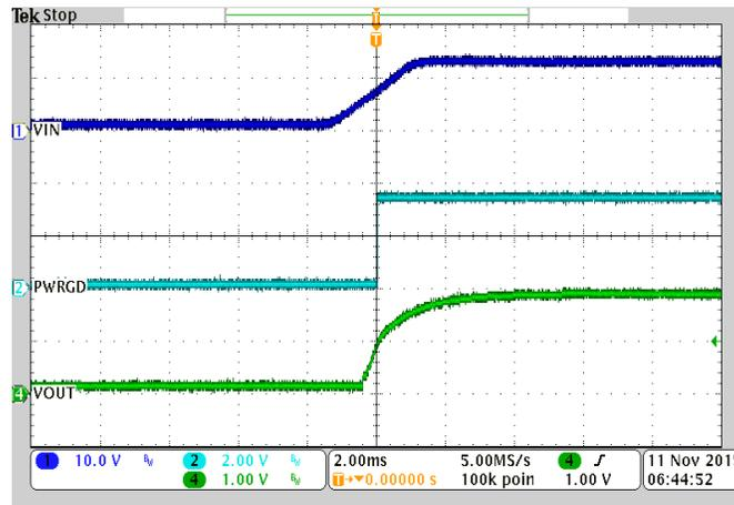
Fig. 17 Start-Up Waveforms for THPM4401A
