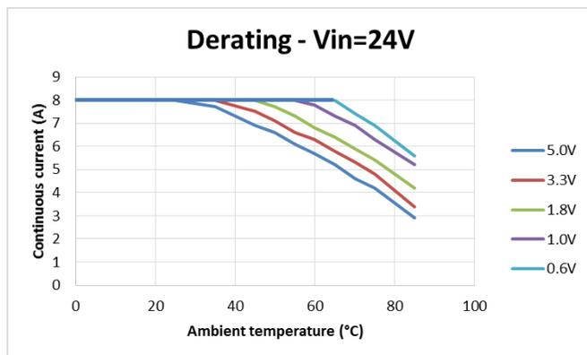
Fig. 31 Output current derating (24V input)
