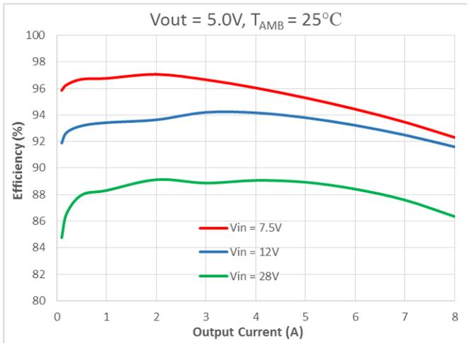
Fig. 3 Efficiency vs Output Current (V<sub>OUT</sub>=5V)
