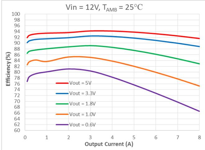
Fig. 1 Efficiency vs Output Current (V<sub>IN</sub>=12V)
