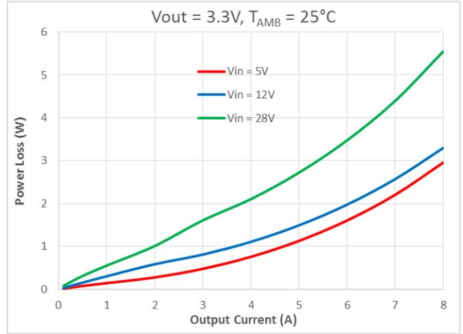
Fig. 6 Power Dissipation vs Output Current (V<sub>OUT</sub>=3.3V)
