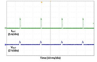
Fig. 38 Recovery from Over-current Shut-down
