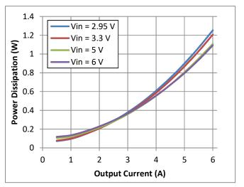
Fig. 10 Power Dissipation vs Output Current
