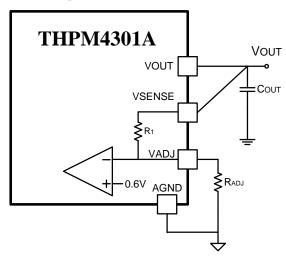
Fig. 15 Output Voltage Setting
