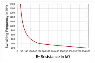
Fig. 33 Switching Frequency Adjustment
