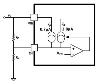
Fig. 28 Input Under-Voltage Lockout Setup
