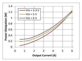
Fig. 4 Power Dissipation vs Output Current
