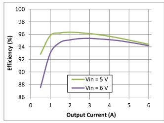
Fig. 1 Efficiency vs Output Current
