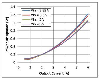
Fig. 12 Power Dissipation vs Output Current
