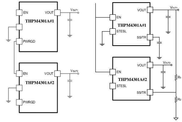
Fig. 29 Sequencing Startup Schematic
