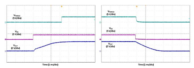
Fig. 26 Waveforms at Enable Turn-On
