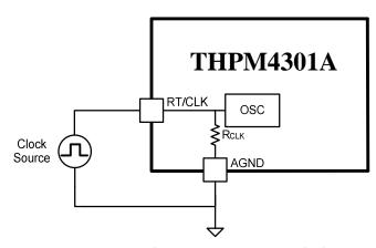
Fig. 35 Synchronizing to a System Clock
