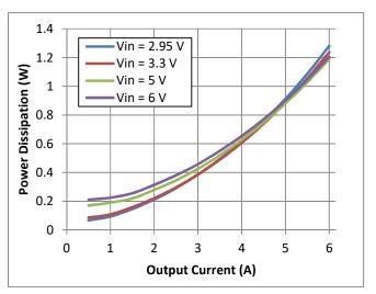
Fig. 6 Power Dissipation vs Output Current
