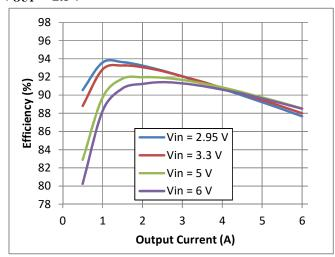
Fig. 7 Efficiency vs Output Current
