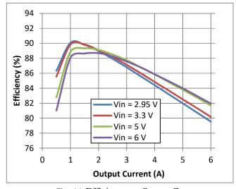
Fig. 11 Efficiency vs Output Current
