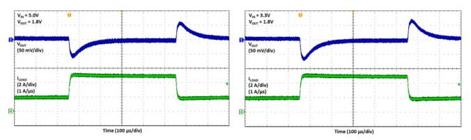
Fig. 20  $V_{IN} = 5V$ ,  $V_{OUT} = 1.8V$ , 3A Load Step
