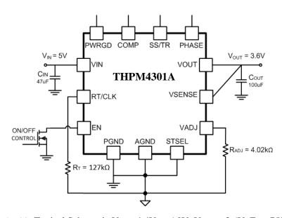
Fig. 23 Typical Schematic  $V_{\rm IN}$  = 4.4V to 6.0V,  $V_{\rm OUT}$  = 3.6V,  $F_S$  = 750kHz
