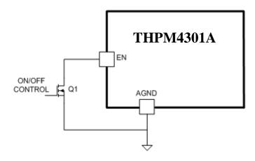
Fig. 25 Typical ON/OFF Control Schematic
