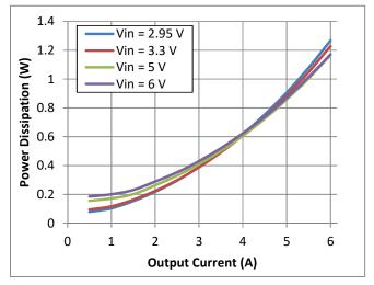
Fig. 8 Power Dissipation vs Output Current
