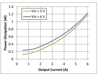
Fig. 2 Power Dissipation vs Output Current
