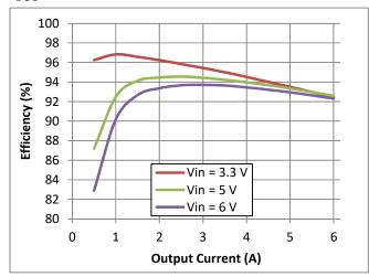
Fig. 3 Efficiency vs Output Current
