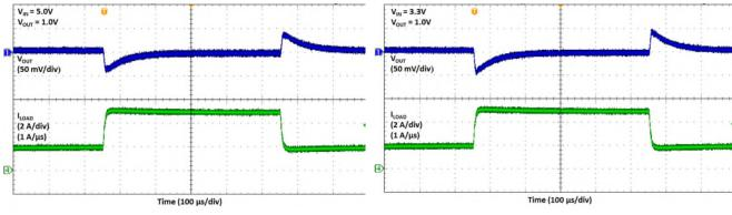
Fig. 16  $V_{IN} = 5V$ ,  $V_{OUT} = 1.0V$ , 3A Load Step
