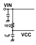
Fig. 1 Filter setup of VCC input
