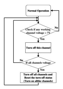
Fig. 3 LED short protection circuit function
