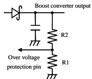
**Fig. 2 Over voltage protection setup**
