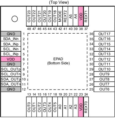
\* The exposed pad is connected to GND inside the device. The exposed pad should be soldered to GND on the PCB.
