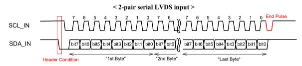
\* The 3-wire to 2-pair bridge function can convert 3-wire serial output from the host such as micro-controller or CPU to 2-pair sereal LVDS. Please refer to the section "3-wire to 2-pair bridge function" for details.
