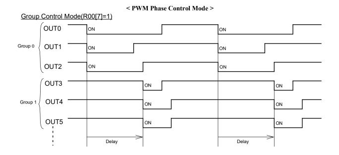
When multiple LED output channels need to be connected in parallel to drive, the PWM phase control mode must be set to group control mode (R00[7]=1), and the channels in the same group must be connected in parallel to drive.
