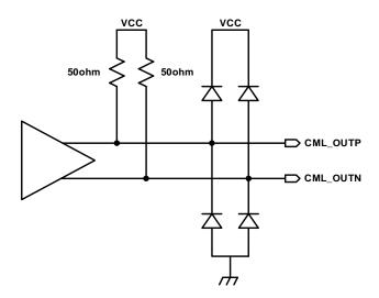
Figure 2. CML Output Schematic Diagram
