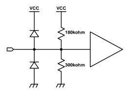
Figure 4. 3-Level Input Schematics Diagram
