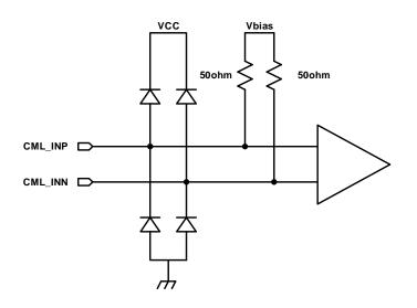
Figure 1. CML Input Schematic Diagram
