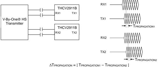
Figure 6. CML Propagation Delay Timing
