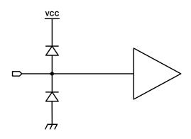
Figure 3. LVCMOS Input Schematics Diagram
