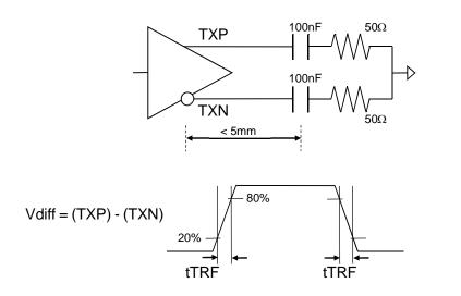
Figure 7. CML Output Switching Timing and Test Circuit
