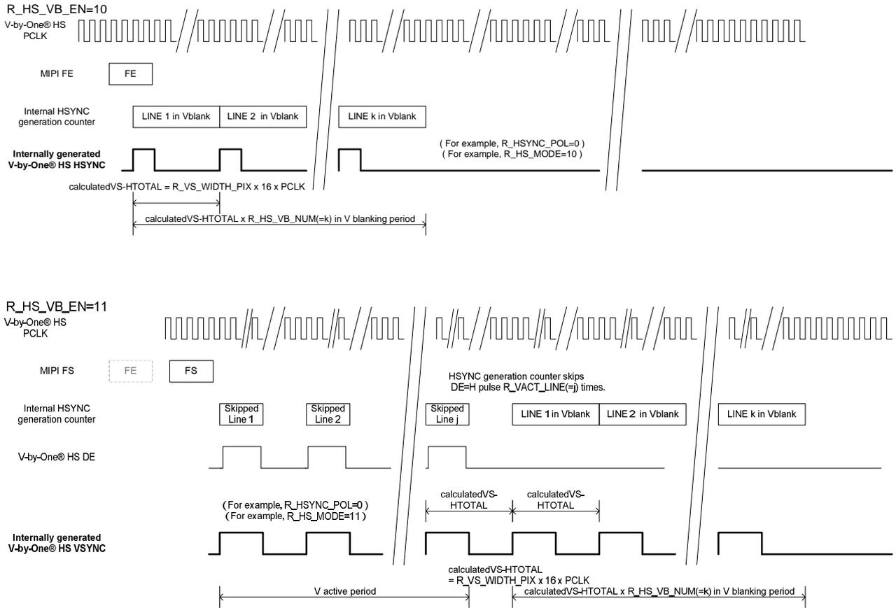
Figure 10. Internally generated HSYNC in Vertical blanking period
