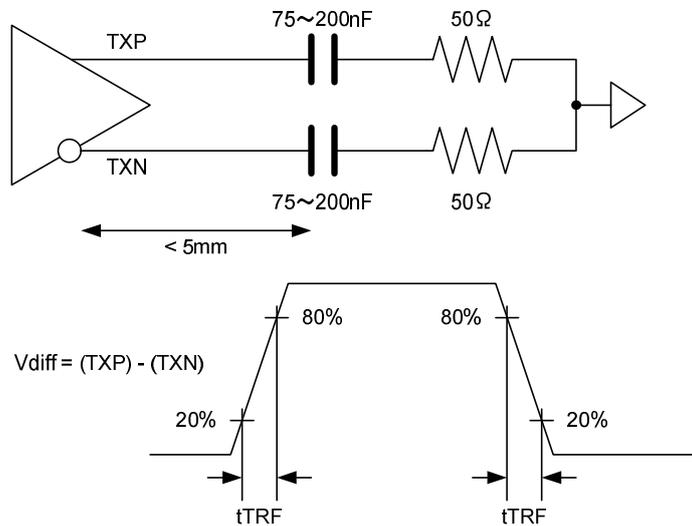
Figure 25. CML Transmitter t<sub>TRF</sub>
