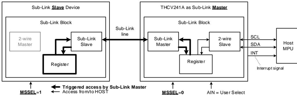
Figure 16. Host MPU to Sub-Link Slave Register via THC241A access configuration
