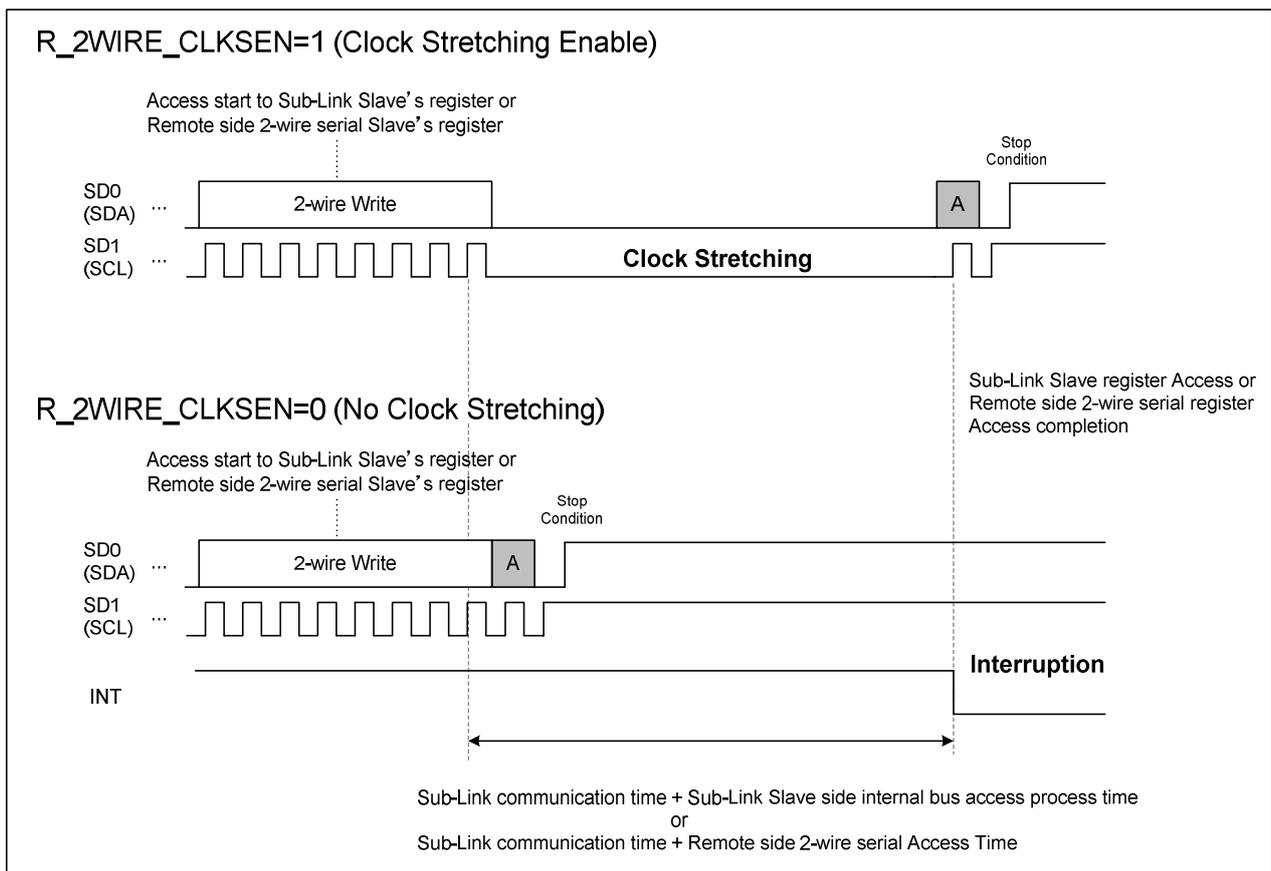
Figure 18. Sub-Link Master 2-wire slave clock stretching operation
