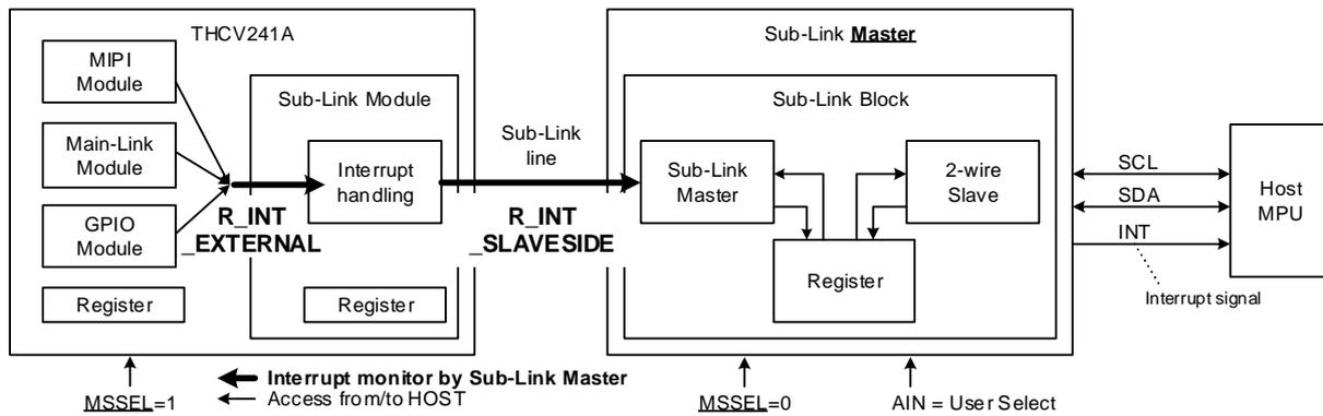
Figure 20. Interrupt configuration external of Sub-Link module.
