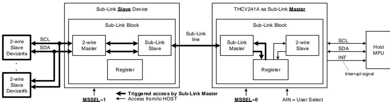
Figure 17. Host MPU to 2-wire slave devices connected to Sub-Link Slave via THC241A access configuration
