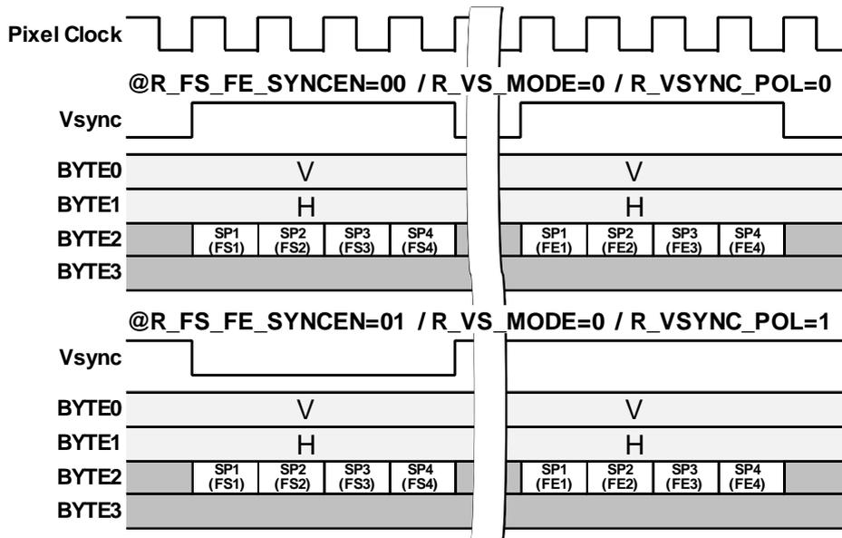
Figure 11. MIPI Short Packet V-by-One® HS bridge timing
