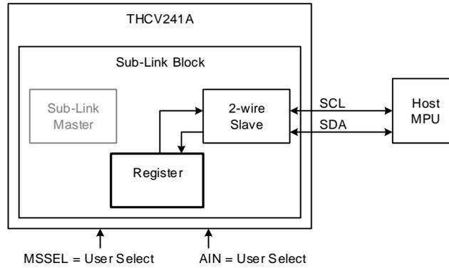
Figure 13. Host to THCV241A local register access configuration
