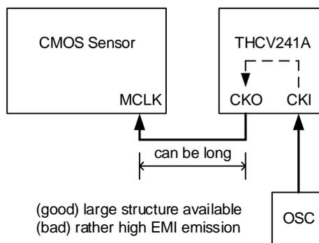
Figure 2. Reference clock supply clock buffer method (optional)
