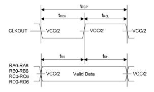
Figure 9. LVCMOS Output Setup and Hold Time
