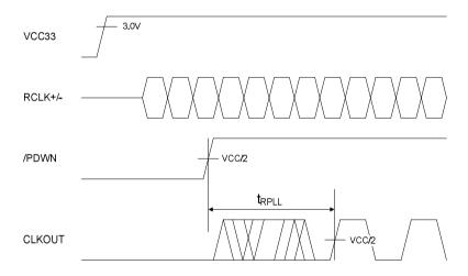
Figure 11. PLL Lock Loop Set Time
