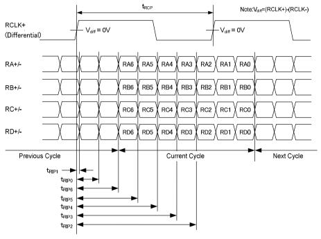
Figure 7. LVDS Input Data Position
