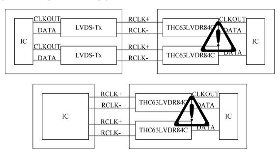
Figure 14. Asynchronous Use
