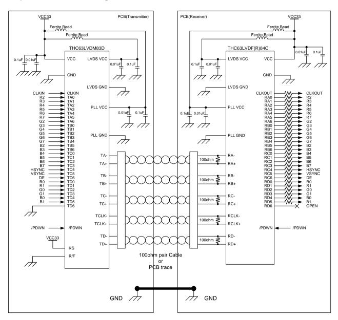
Figure 12. Connection Example with JEIDA Format
