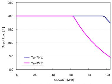
Figure 6. LVCMOS Output Load Limitation
