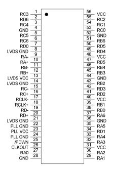
Figure 2. Pin Diagram
