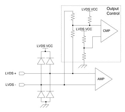
Figure 3. LVDS Input Schematic Diagram
