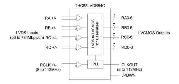
Figure 1. Block Diagram
