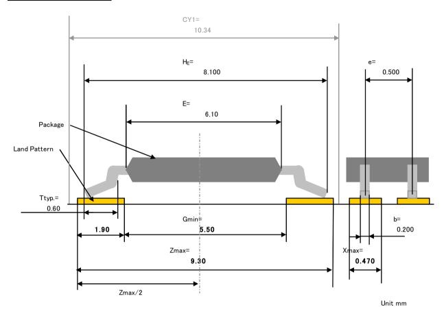
The recommendation mounting method of THine device is reflow soldering. The reference pattern is using the calculation result on condition of reflow soldering.
