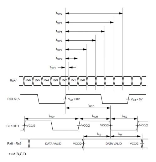
Data and Clock Input to Output AC Timing Diagram
