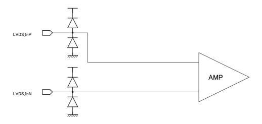
**LVDS Input Schematic Diagram**
