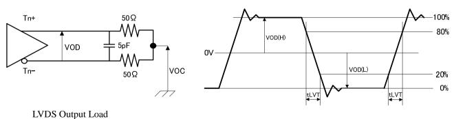
Figure 6. LVDS Output Load and Transmission Time
