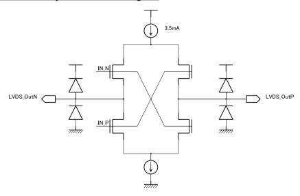
Figure 3. LVDS Output Schematic Diagram
