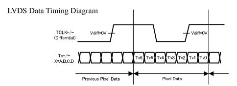
Figure 12. LVDS Data Timing Diagram
