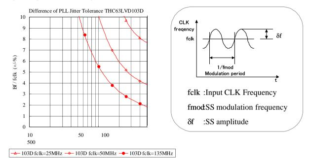
Figure 11. Spread Spectrum Clocking Tolerant
