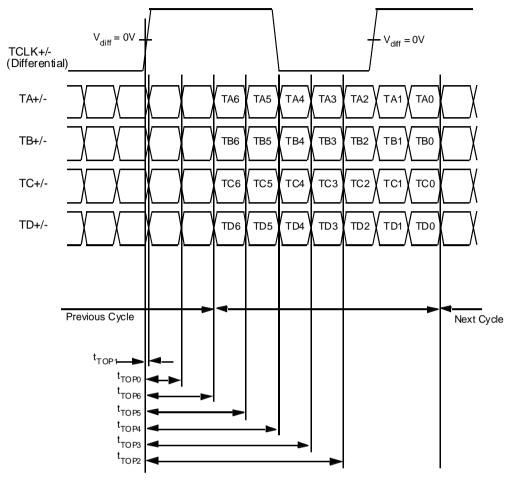
**Figure 9. LVDS Output Data Position**
