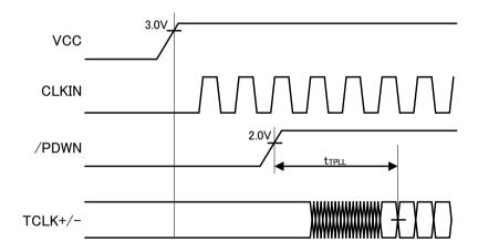
Figure 10. PLL Lock Loop Set Time
