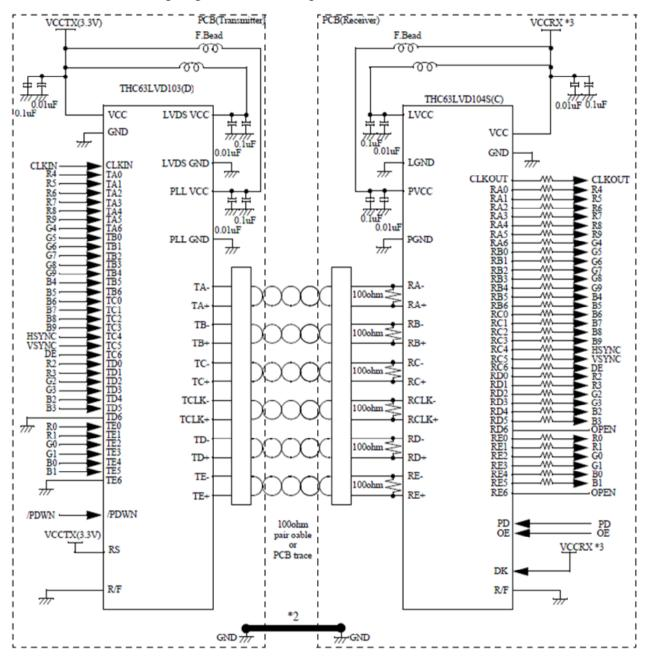
**Figure 13. Typical Connection Diagram**
