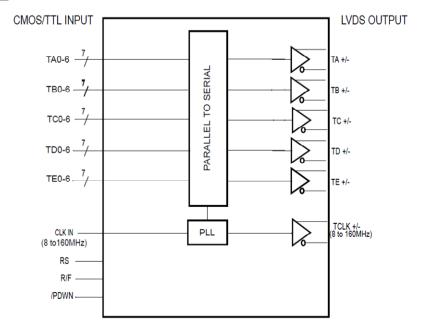
Figure 1. Block Diagram
