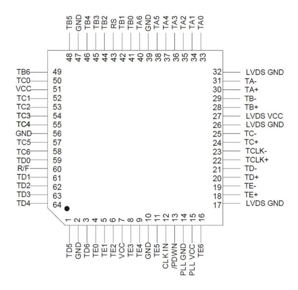
Figure 2. Pin Diagram
