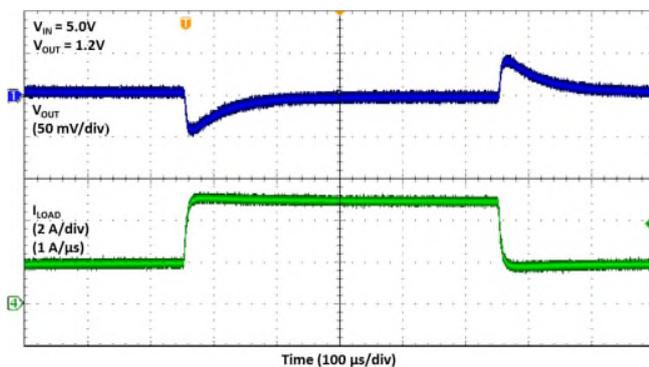
Fig. 18  $V_{IN} = 5V$ ,  $V_{OUT} = 1.2V$ , 3A Load Step
