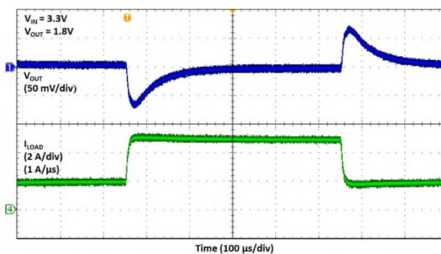
Fig. 21  $V_{IN} = 3.3V$ ,  $V_{OUT} = 1.8V$ , 3A Load Step
