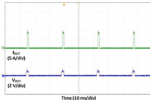
Fig. 39 Hiccup Mode Current Limit Restart into Short-Circuit
