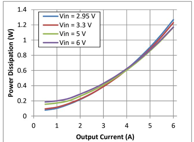
Fig. 8 Power Dissipation vs Output Current
