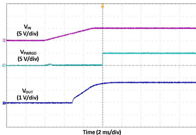
Fig. 24 Startup Waveforms
