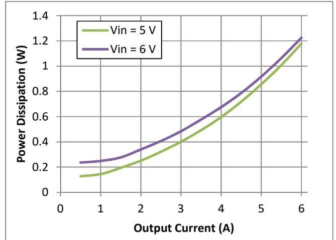
Fig. 2 Power Dissipation vs Output Current
