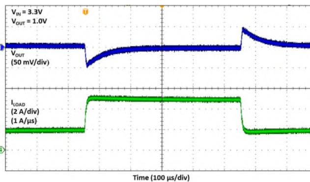
Fig. 17  $V_{IN} = 3.3V$ ,  $V_{OUT} = 1.0V$ , 3A Load Step
