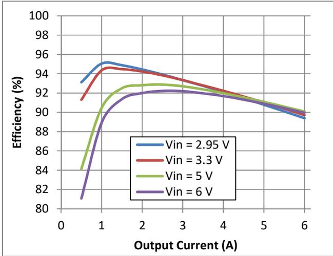
Fig. 5 Efficiency vs Output Current
