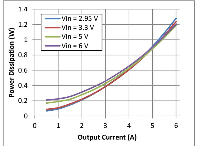
Fig. 6 Power Dissipation vs Output Current
