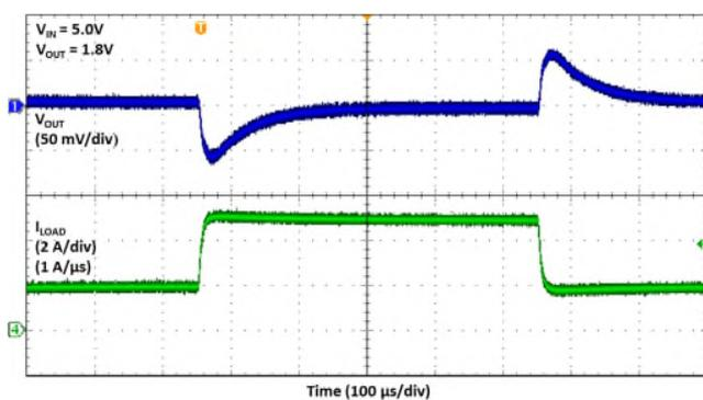
Fig. 20  $V_{IN} = 5V$ ,  $V_{OUT} = 1.8V$ , 3A Load Step
