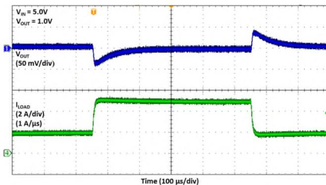
Fig. 16  $V_{IN} = 5V$ ,  $V_{OUT} = 1.0V$ , 3A Load Step
