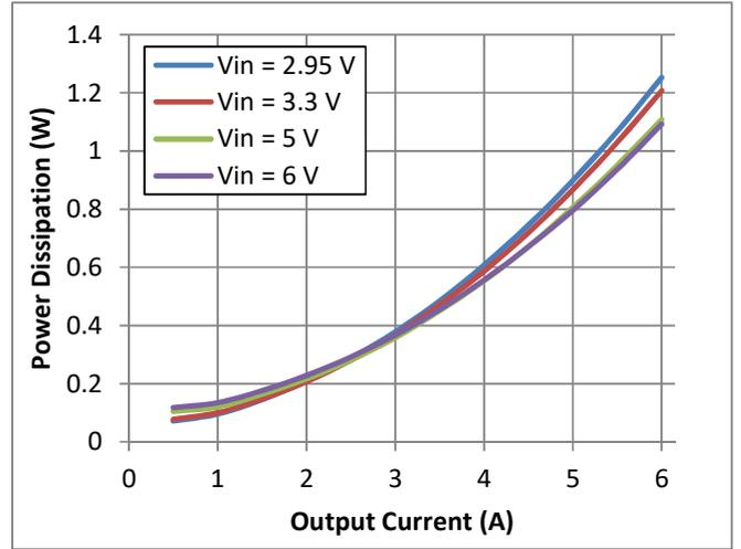
Fig. 10 Power Dissipation vs Output Current
