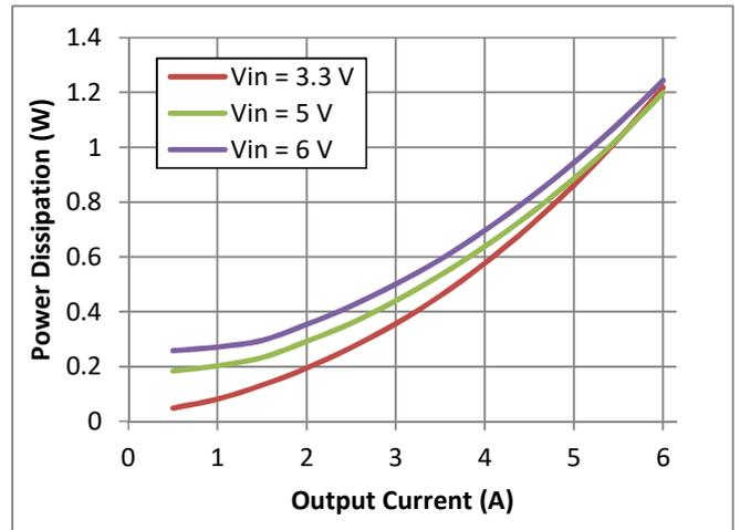
Fig. 4 Power Dissipation vs Output Current
