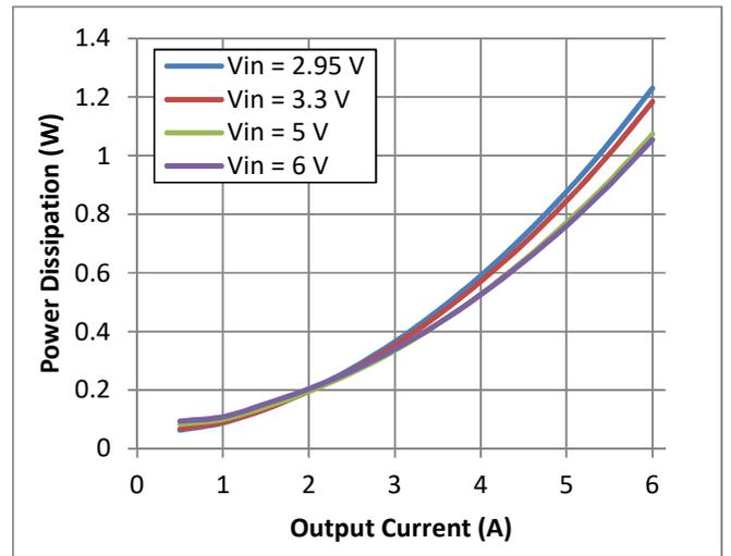
Fig. 12 Power Dissipation vs Output Current
