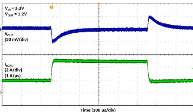
Fig. 19  $V_{IN} = 3.3V$ ,  $V_{OUT} = 1.2V$ , 3A Load Step
