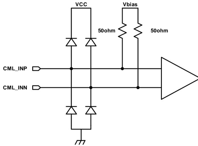
**Figure 1. CML Input Schematic Diagram**
