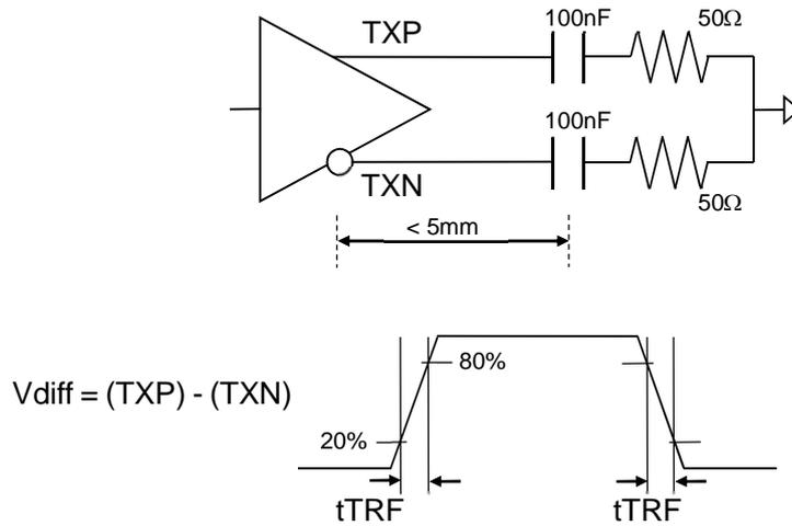
**Figure 7. CML Output Switching Timing and Test Circuit**
