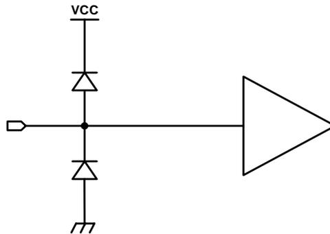
**Figure 3. LVCMOS Input Schematics Diagram**
